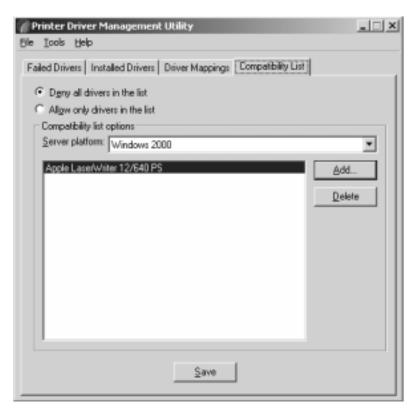
**Deny list** – All drivers except those in the list are allowed to be installed on the application server. If a client tries to install a denied driver, an entry is made to the event log by the application server.
